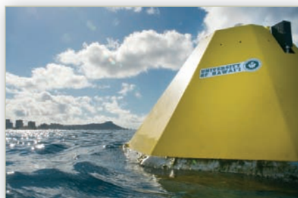
NOAA's Pacific Marine Environmental Lab (PMEL) works with the regions on their ocean acidification monitoring programs. This buoy in Hawaii is jointly funded by PMEL and IOOS® and includes CO 2 sensors. This is an example of a single observing system serving multiple purposes. (R. David Beales, University of Hawaii Creative Services)
