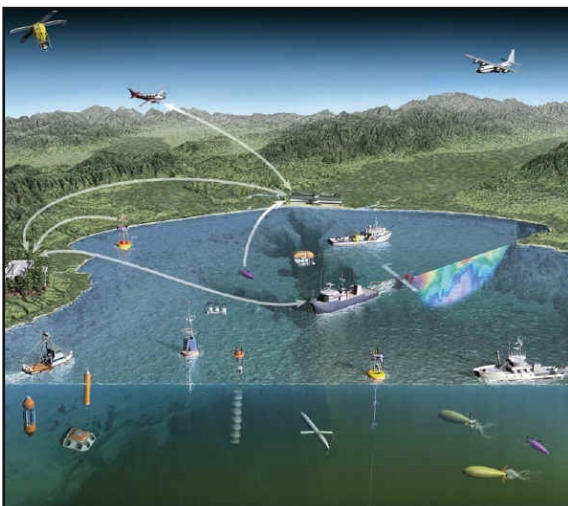
Figure 3.1. Adaptive coastal sampling: Coordinated, synergistic use of multiple remote and in situ assets
