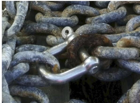
Galvanic corrosion caused by pairing stainless steel with galvanized chain. More info can be found on [this helpful rigging website](#).
